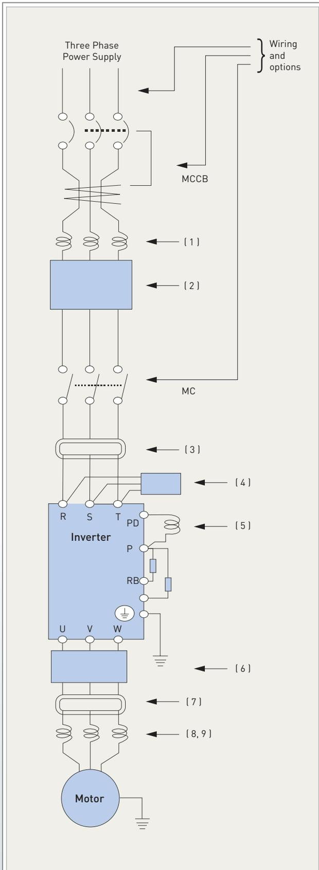
The sensitivity of circuit breaker (MCCB) should be differentiated by the sums of wiring distances (inverter-power supply and inverter-motor).
