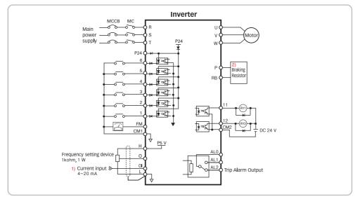
1) In case of changing terminal No.5 to No. 13 AT(current input selection) on : 4~20mA selection / off : Volume selection
